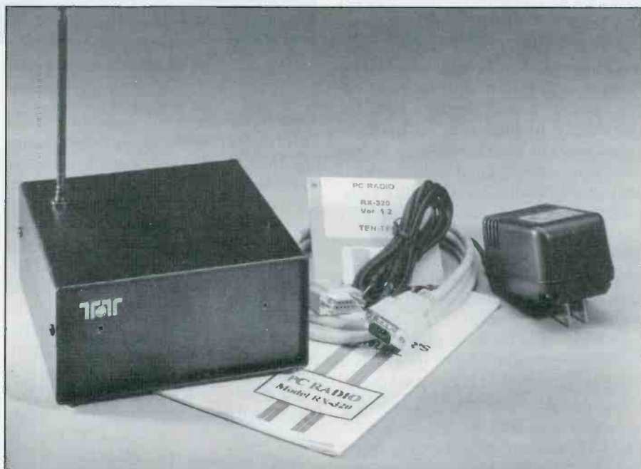
At left is the RX-320 receiver. Also shown are the manual, cables, software disk, and 12-vdc wall power pack.
